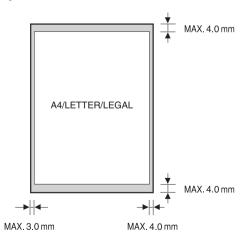
The margin at each edge is outside the machine's scanning area.
